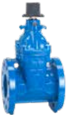
Series 45/59 Flanged gate valve with wrench nut DN50, 250 and 300 17.2 bar (250 PSI) PN16 drilling Ductile iron UL/ULC listed, FM approved
