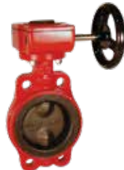
Series 75 Butterfly valve Centric with fixed liner Semi lug DN50-300 PN10/16 Ductile iron FM approved
