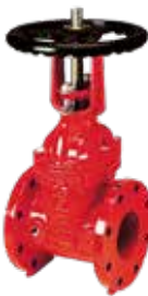
Series 45/56 Flanged gate valve with rising stem OS&Y DN50-300 17.2 bar (250 PSI), UL/ULC listed, FM approved DN350-400 13.7 bar (200 PSI), UL/ULC listed 17.2 bar (250 PSI), FM approved PN16 drilling. Ductile iron
