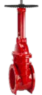
Series 55 Flanged gate valve with rising stem OS&Y DN450-600 13.7 bar (200 PSI), UL/ULC listed 17.2 bar (250 PSI), FM approved PN16 drilling 316 stem Ductile iron
